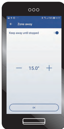
Away mode: Set "Away" mode temperature until you manually stop the settings.
